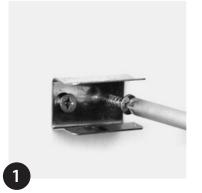
Fix clips with suitable screws (min 3 clips per metre or every 500mm/20").
